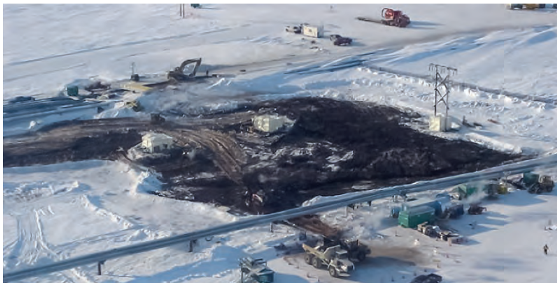
Figure III-1.4 Spill from a pipeline leak onto tundra near the coast in winter. The oil has been exposed by removal of the uniled surface snow (Source: Alaska Clean Seas).
