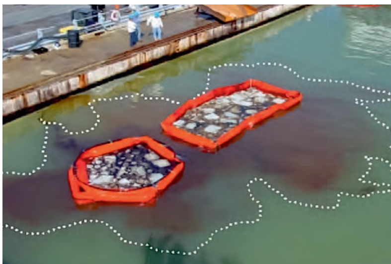
Figure V-4.3 View of successful dispersion occurring with oil in simulated broken ice (Sources: Owens and Belore (2004), Aker Arctic).
