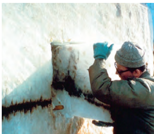
Figure IV-1.6 Cut out of a large ice block removed from an under ice spill on the North Slope of Alaska, showing the encapsulated oil layer with new ice growth beneath the oil (Photo: A. Allen).
