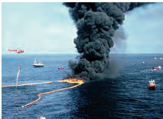
Figure V-5.3 Open water burning of crude oil in a fireproof boom after ignition with a Helitorch during the Newfoundland Offshore Burn Experiment in 1993 (Source: Environment Canada).
