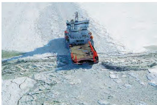
Figure V-4.3 View of successful dispersion occurring with oil in simulated broken ice (Sources: Owens and Belore (2004), Aker Arctic).
