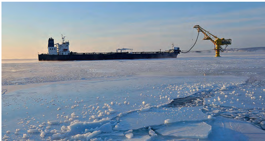
Figure C.4 Single point mooring with Tanker loading oil from Sakhalin 1 at the De Kastri terminal.
