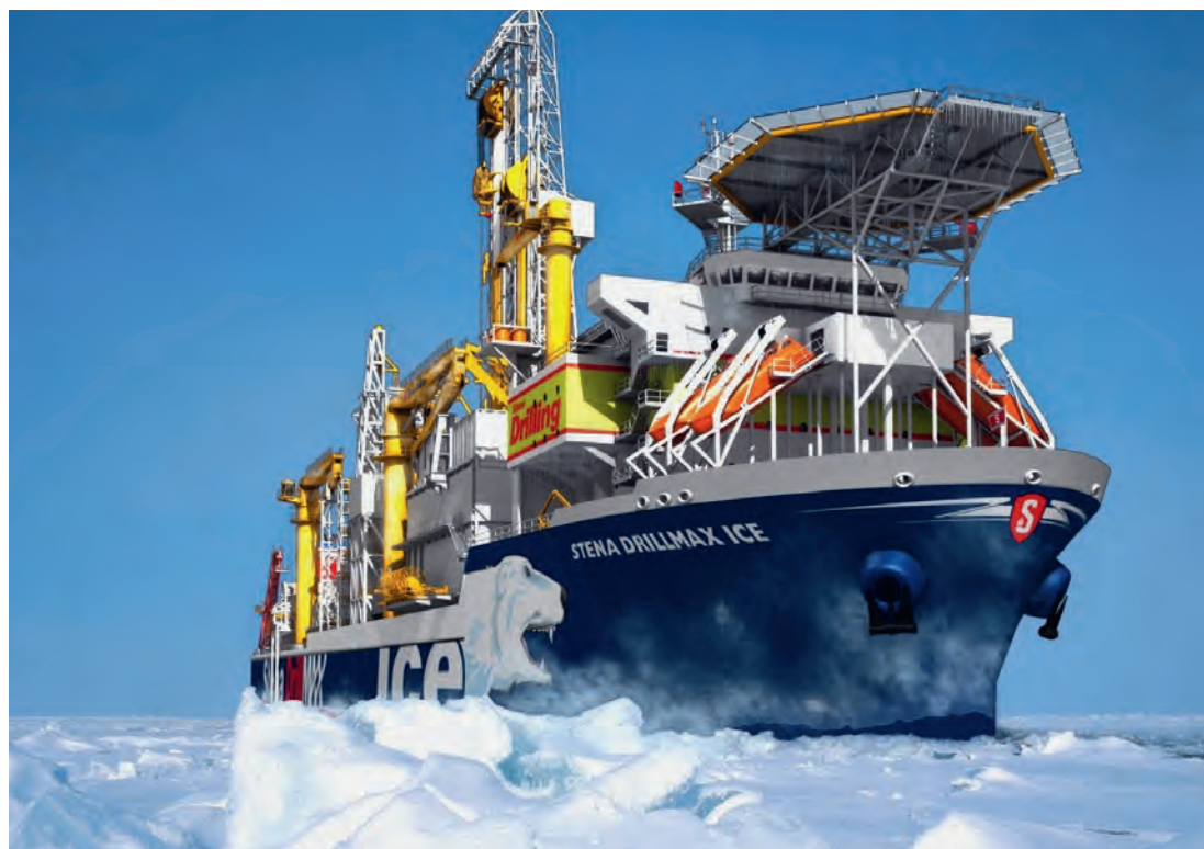
Figure C.2 Stena Drillmax Ice, an example of a modern Arctic, ice class drillship (Illustration: Stena).
