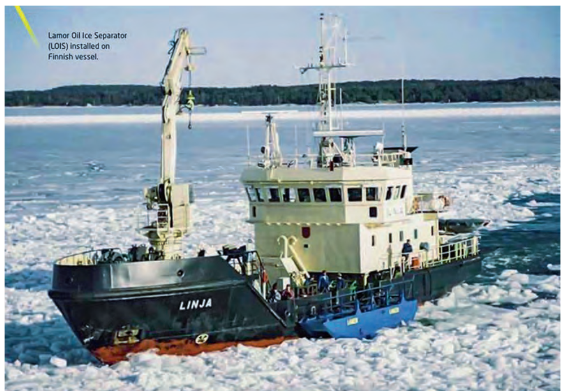
Figure V-3.3 Finnish OSRV Linja with the LOIS vibrating grid oiled ice cleaners mounted on either side in collecting mode. This view clearly shows the limited swath width possible with these systems (Photo: Lamor Newsreel, 2011).
