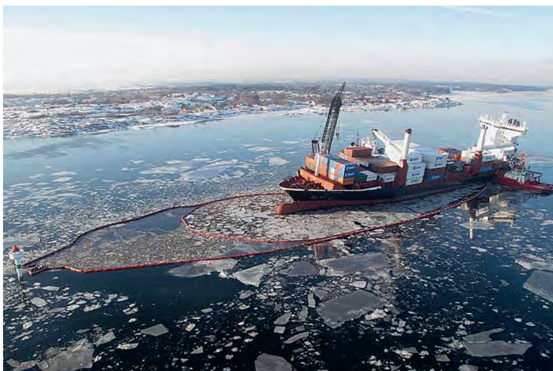
Figure E.4 Boom surrounding the Godafoss casualty in the ice-covered waters of the Ytre Hvaler National Marine Park, Norway (Photo: ITOPF).
