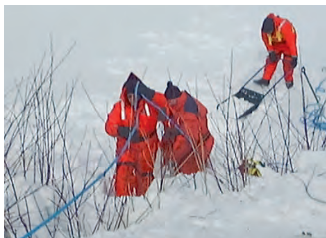
Figure VI-1.3C Snow removal to detect subsurface oil in snow (Source: ECRC).
