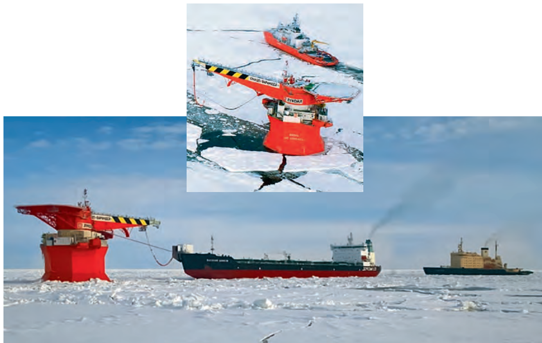
Figure III-1.2 Tankers loading in ice at the Russian Varandey offshore terminal with support icebreakers in attendance.
