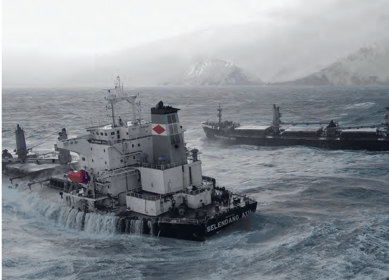
Figure E.3 MV Selendang Ayu broken into two halves after grounding off Unalaska Island (Photo: US Coast Guard).
