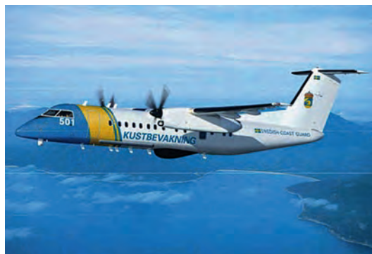
Figure V-2.2 Swedish Q300 aircraft representative of the state of the art in open water maritime pollution surveillance (Photo: Swedish Coast Guard).
