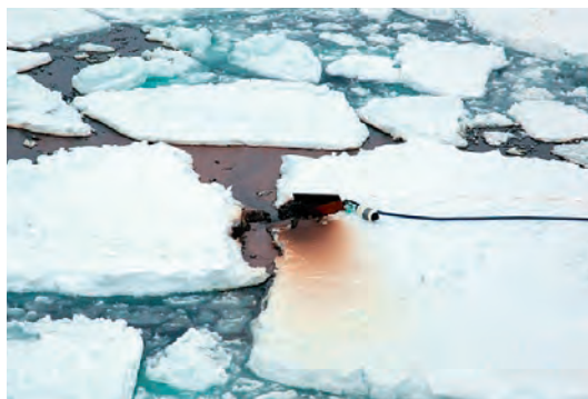
Figure IV-1.5 View of the main 59 bbl (7 cubic metre) spill in 8/10 pack ice while being discharged during the 2009 SINTEF Oil in Ice field experiment in Svalbard, Norway. The effectiveness of the closely packed floes in trapping and containing the oil in this situation is clearly apparent. Very little additional spreading occurred in subsequent days (Photo: SINTEF).
