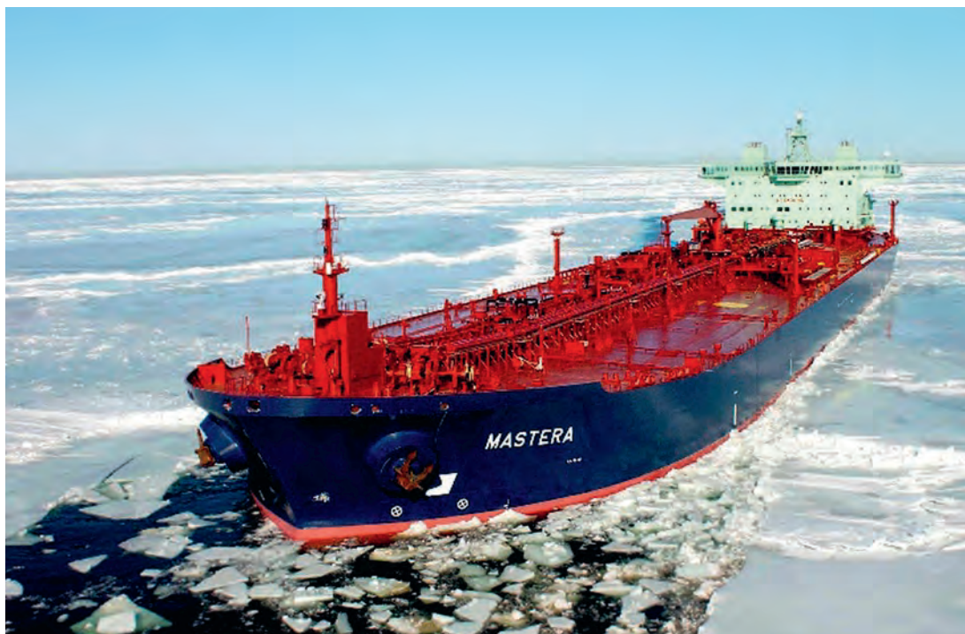
Figure E.1 MT Mastera (106,000 DWT) operating in the Baltic. Delivered in 2003 as the first commercial ship to utilize the Double Acting Tanker (DAT) concept. The Mastera and her sister vessel Tempera represents the current generation of ice-going tanker design with double hulls, ice strengthening Baltic 1A Super, and the most advanced spill prevention systems (Photo: Aker Arctic).
