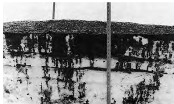
Figure IV-1.10 Cross-section sketch and photograph of cold oil spill on snow. The oil drained through the surface snow and accumulated above the layers of ice (from Mackay, 1974).
