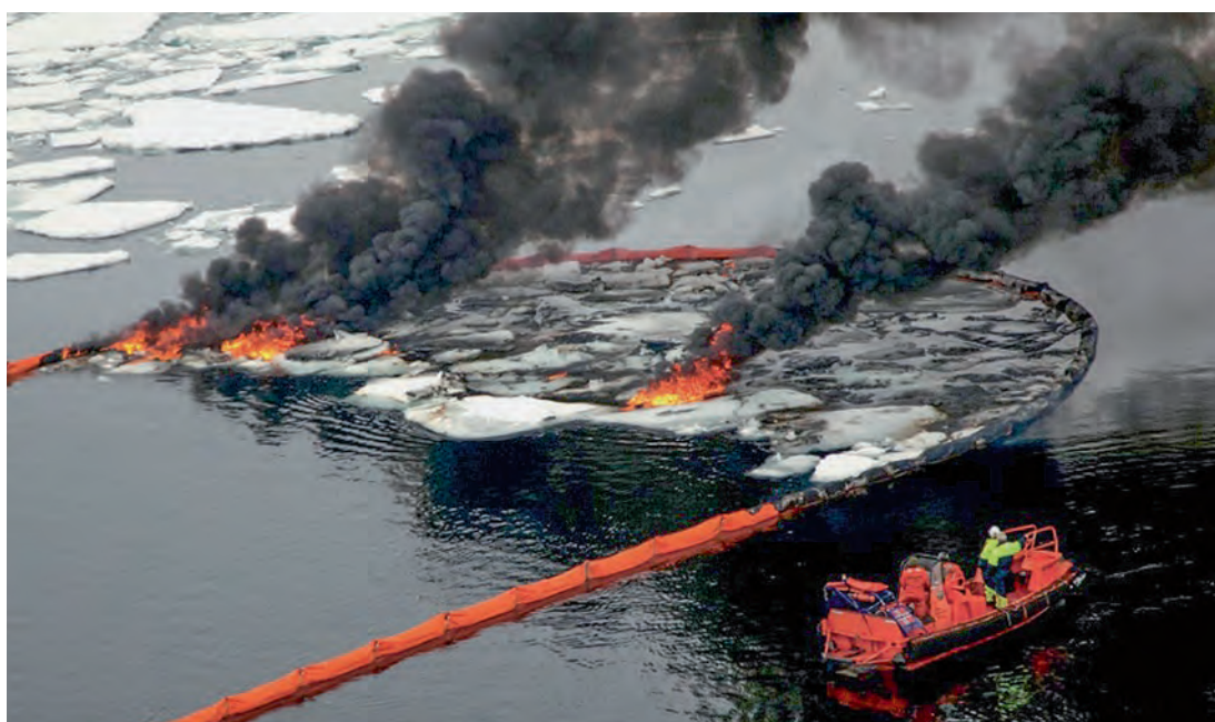
Figure V-5.2 Burning crude oil spilled into a field of small ice cakes collected in a fire-resistant boom – Norway 2009 (Potter et. al 2012).
