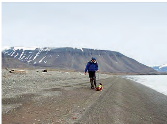
Figure VI-1.2 Dog detection team locating buried oil on an arctic shoreline— Svalbard (Source: SINTEF).
