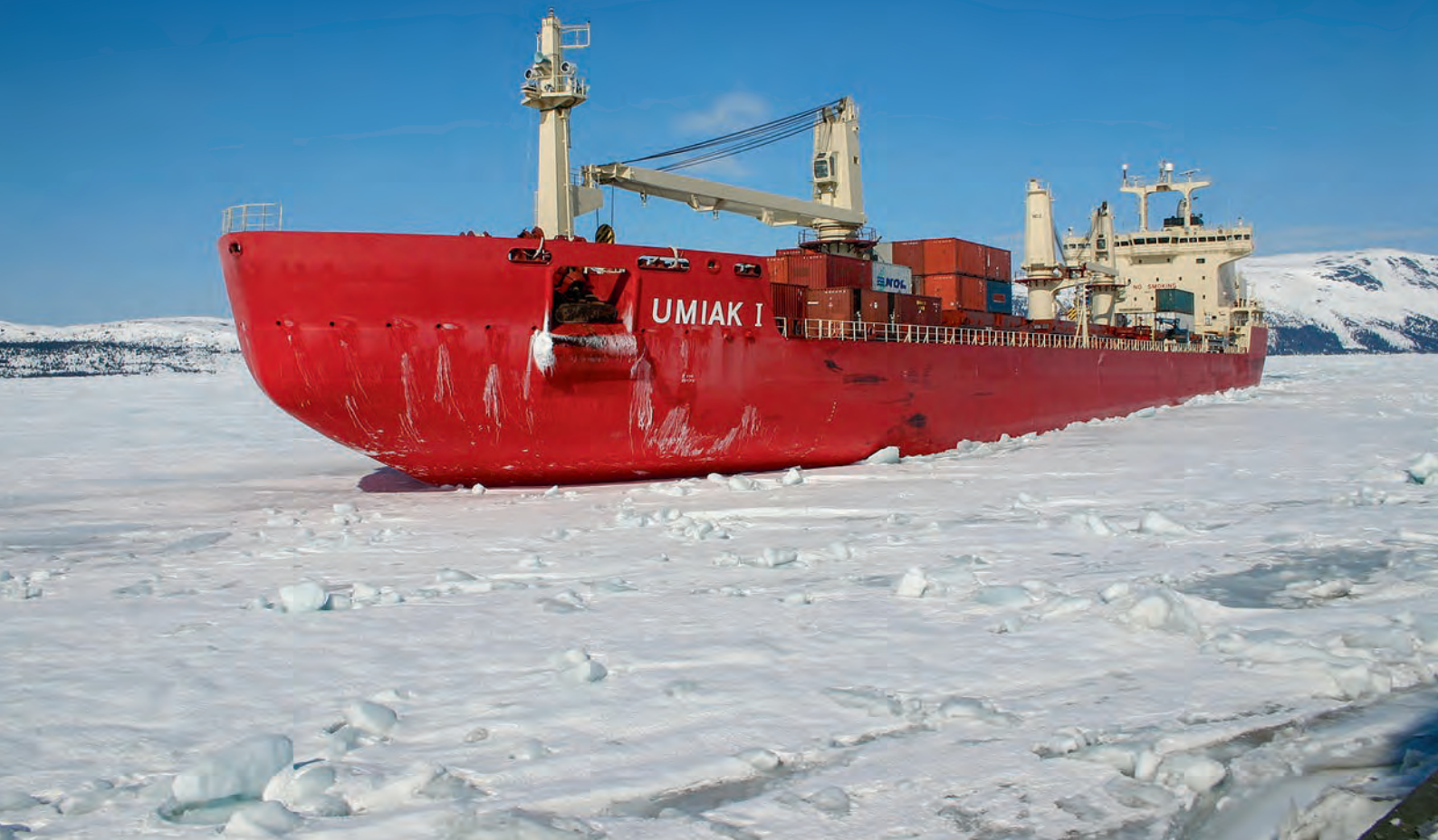
Figure III-1.1 Polar Class 4 icebreaking Canadian ore carrier Umiak, serving mines in northern Quebec and Labrador. This vessel and her sister ship the Nunavik are among the most advanced and capable ice-going commercial cargo vessels currently operating in the Arctic (Source: CNW Group/Fednav Limited).
