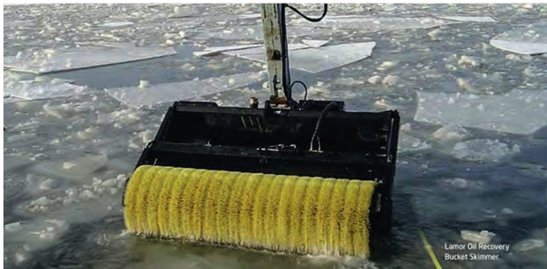
Figure V-3.2 Close-up of the brush bucket skimmer operating in ice (Source: Lamor Newsreel).
