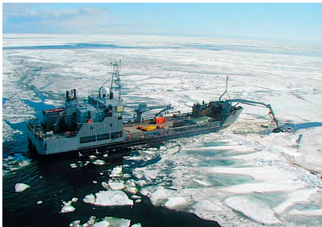
Figure V-3.1 Hylje Finnish oil spill response vessel using an over-the-side brush bucket on a hydraulic arm (see close-up below) to recover oily bilge pumped illegally into the winter shipping lane in the Baltic in March 2003 (Source: Finnish Environment Institute, SYKE).
