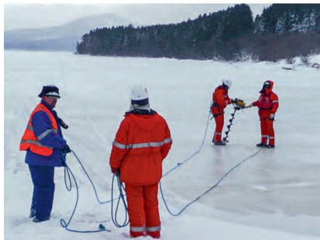
Figure VI-1.3A Drilling through ice to detect subsurface oil (Photo credit: E. Owens).
