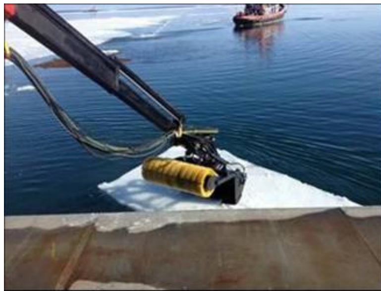
Figure 24. LRB demonstrating ability to push ice out of way.
