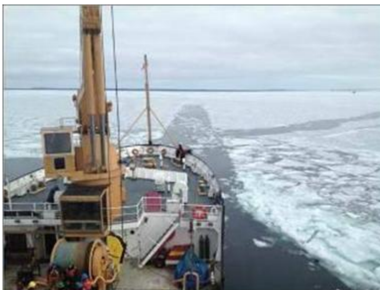
Figure 18. Channel or ‘slot’ created in sheet ice to facilitate oil skimmer deployment.
