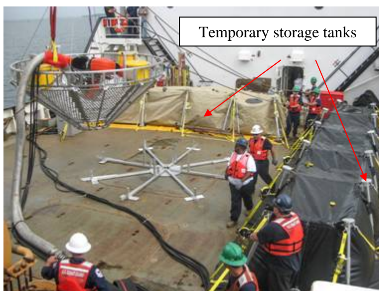
Figure 5. Two temporary storage tanks fully erected on the deck during the underway demonstration.
