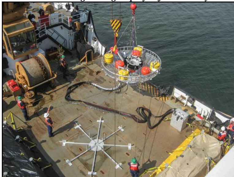
Skimmer with Ice Cage Being Deployed from a Buoy Tender
