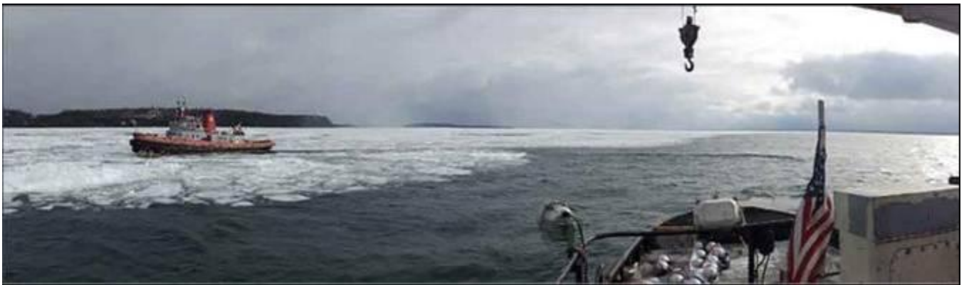
Figure 26. PyroBoom deployed and towed by two tugboats to simulate collection of oil in rubble ice.
