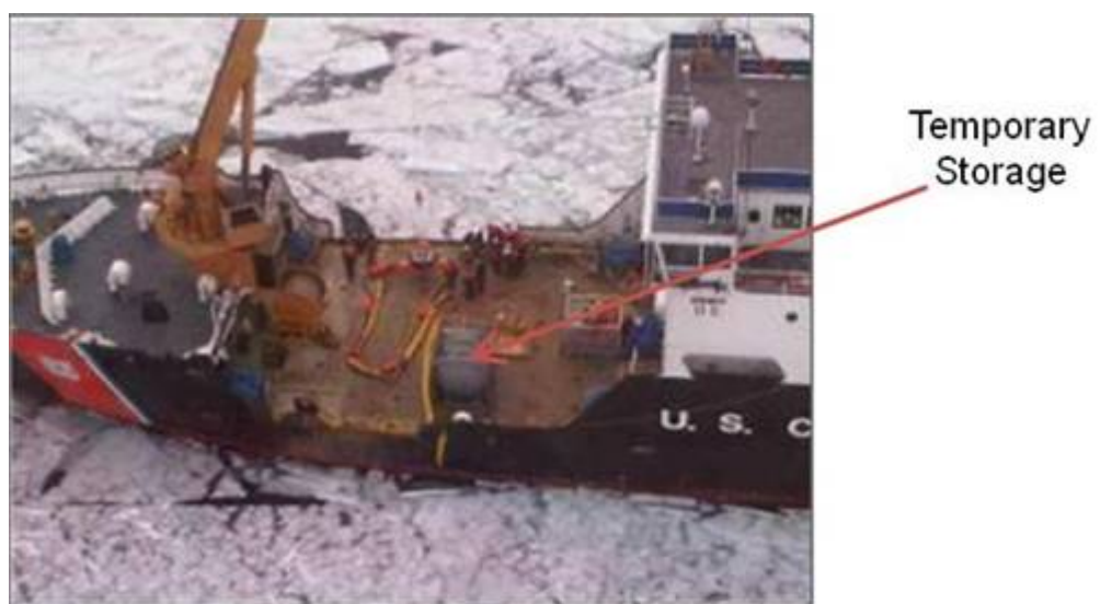
Figure 3. A temporary storage container mid-deck on a Juniper Class Seagoing WLB.
