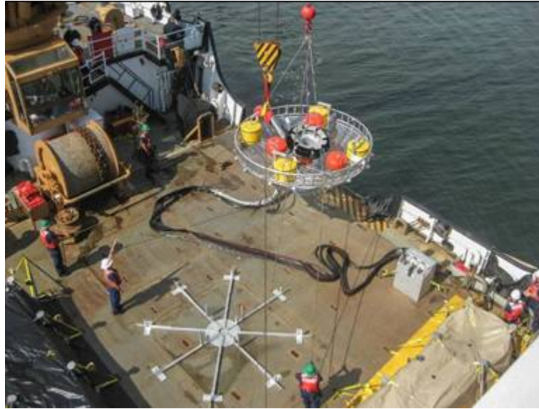
Figure 8. Ice cage integrated with a DOP-Dual Helix skimmer.
