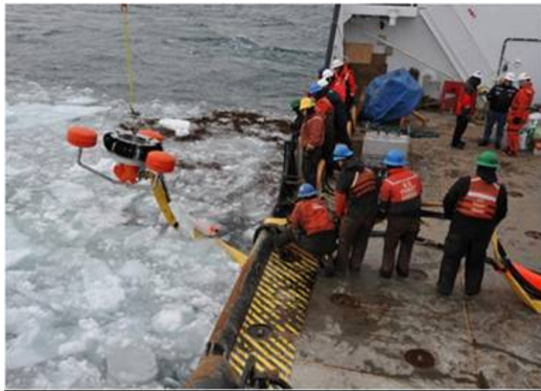
Figure 1. CG buoy tender deployment of SORS skimmer.
