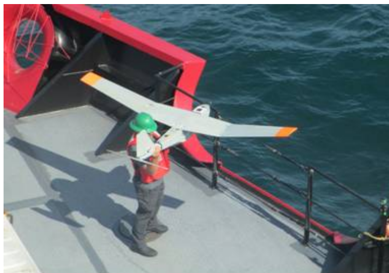
Figure 12. SUAS being deployed from the CGC Healy .
