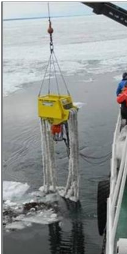
Figure 20. Rope mop skimmer deployed in open water pocket.
