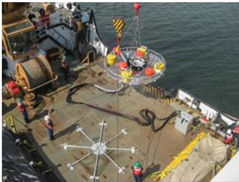
Figure 25. Ice Cage being deployed with DOP Dual Helix skimmer.
