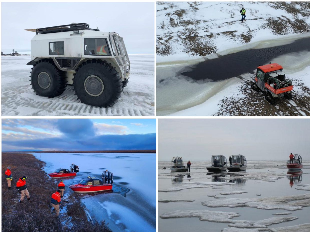
Figure 4-3. Examples of airboats and amphibious vehicles used to access areas of water and thin ice. Clockwise from top left, SHERP, Kubota ATV with tracks, airboats (open and closed cab), and Husky airboats. Photos: ACS.
