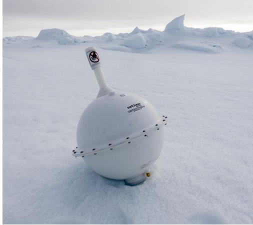
Figure 5-5. Positioning buoy deployed on Arctic Sea ice. Photo: Alfred Wegener Institute/Mario Hoppmann.
