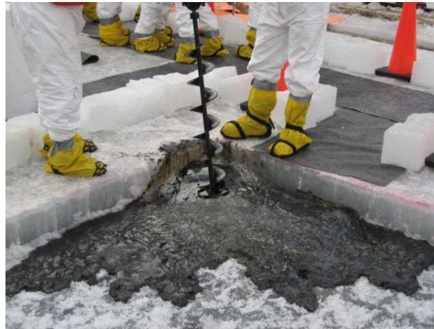
Figure 6-13. Trench and recovery sump cut into ice over an oil pocket. An auger hole is drilled through the ice within the trench or sump, allowing oil to rise through the hole and fill the recovery area. Photo: ACS.
