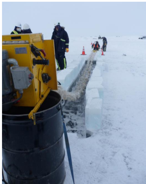
Figure 6-26. Rope Mop skimmer placed in a trench. Photo: ACS.
