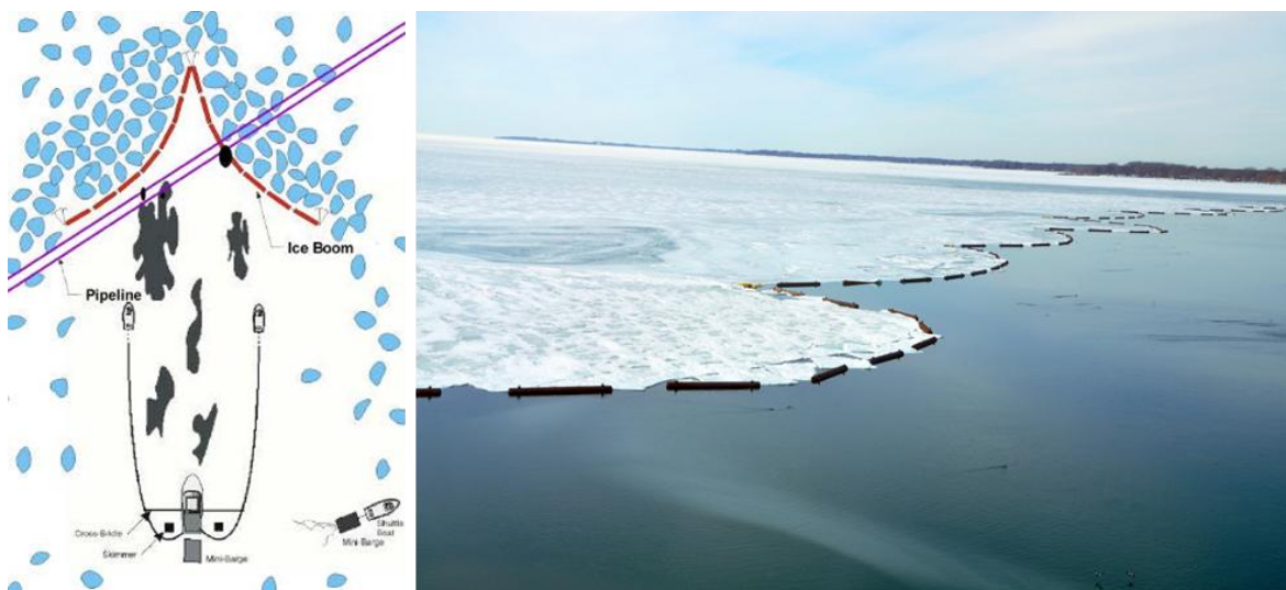
Figure 6-11. (Left) Diversionary ice boom up current of subsea pipeline break. (Right) Lake Erie-Niagara ice boom consists of a 1.7-mile span of floating steel pontoons linked together by steel cables and anchored to the river bottom ( https://www.opg.com/news-and-media/our-stories/story/ice-booms-keep-rivers-flowing/ ).
