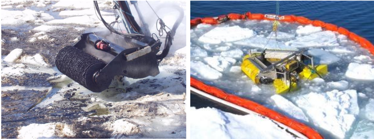
Figure 6-25. (Left) Lamor LRB skimmer recovering oil in ice. Photo: Syke. (Right) Framo prototype self-propelled Arctic skimmer being tested in the Norwegian Barents Sea in 2009. Photo: Ivar Singaas, SINTEF.
