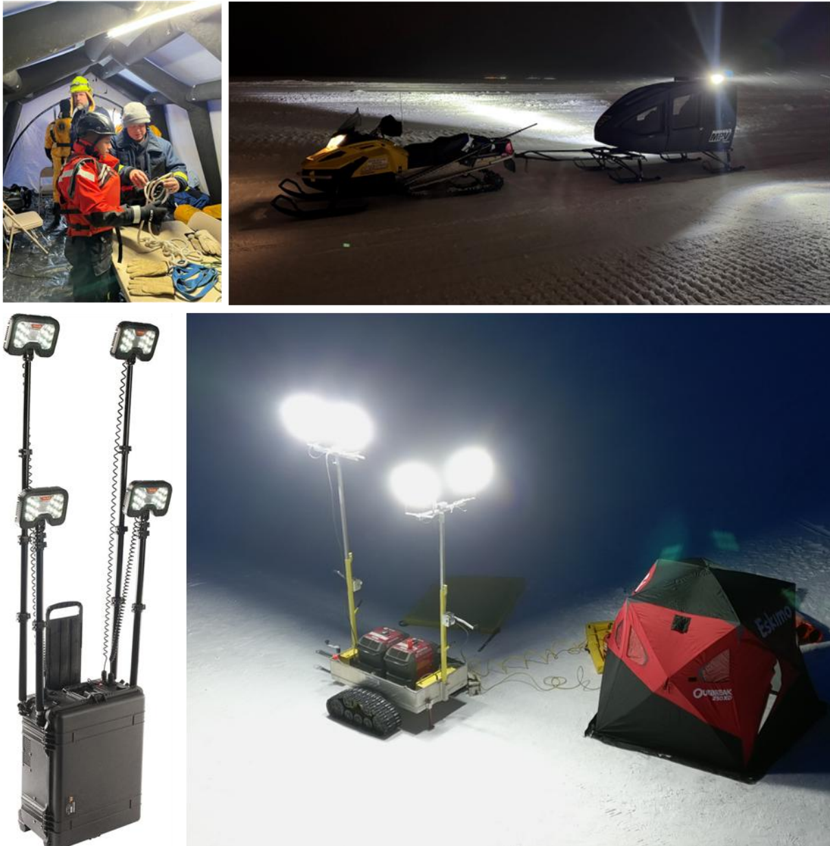
Figure 4-7. Clockwise from top left. Plastic LED tube lamp in Zumro, battery-powered light bar on snow mobile coach exterior, flood lights on tracked trailer with generators, and Pelican remote area battery powered light plant. Photos: ACS.
