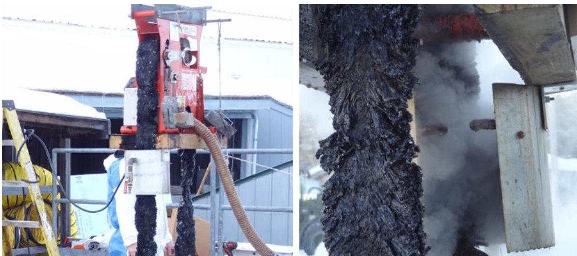
Figure 6-5. (Right) Application of steam to oleophilic surface. (Left) view of adhesion belt. Photos: ACS.
