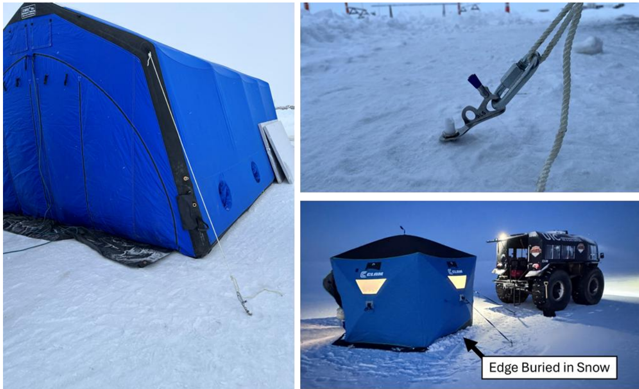
Figure 4-9. Clockwise from left. Zumro Tent with anchor line attached. Ice screw being used as an anchor. Buried edge of ice fishing tent. Photos: ACS.
