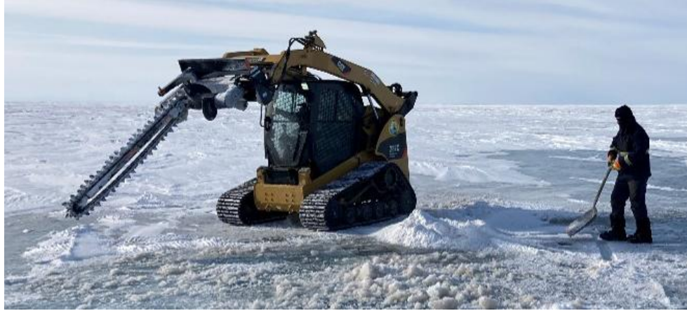
Figure 6-16. 72" trencher attached to skid steer loader. Photo: ACS.
