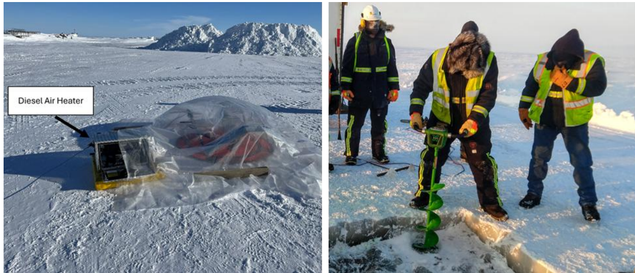
Figure 4-8. (Left) Reinforced plastic sheeting placed over a drone and held down by timbers to keep batteries and internal components warm between flights. Heat source is a diesel air heater. (Right) Battery-powered auger. Photos: ACS.
