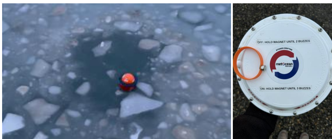
Figure 6-35. Examples of relatively low-cost oil tracking buoys suitable for mild to moderate ice conditions. (Figure 5-5 shows a more robust and costly ice buoy designed for Arctic deployment). Photos: ACS.
