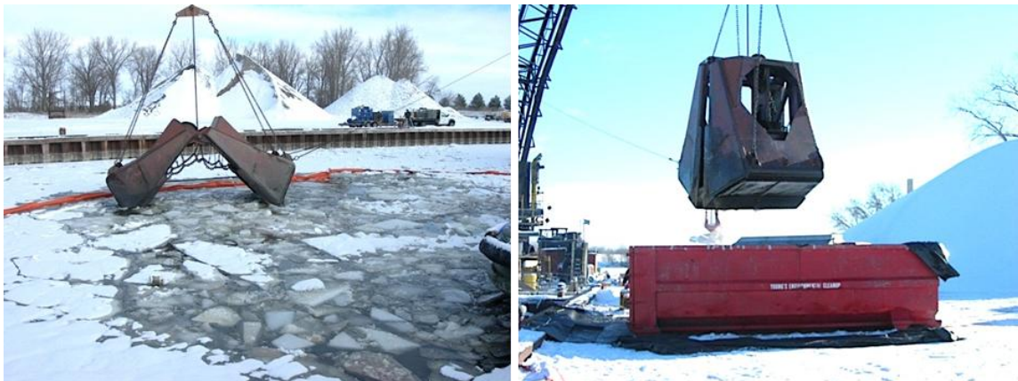
Figure 6-28. Clamshell bucket being used to scoop up oiled ice (left) and deposit it into a lined container (right) for transport to disposal site. Photos: Enbridge.
