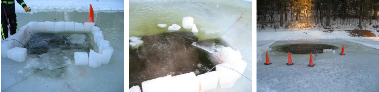
Figure 6-2. Time lapse of velocity jet de-icer deployed in a 5 ft x 6 ft sump cut into a freshwater pond. Times are T=0 (deployment), T+1 hour, T+14 hours (approximately 16 ft diameter hole). Photos: ACS.
