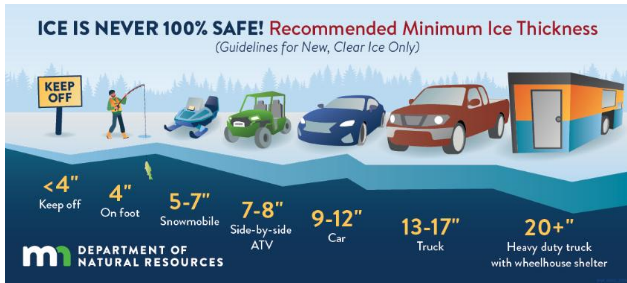
Figure 2-16. Guide to minimum lake ice thickness required to support loads. Source: https://www.dnr.state.mn.us/safety/ice/thickness.html .
