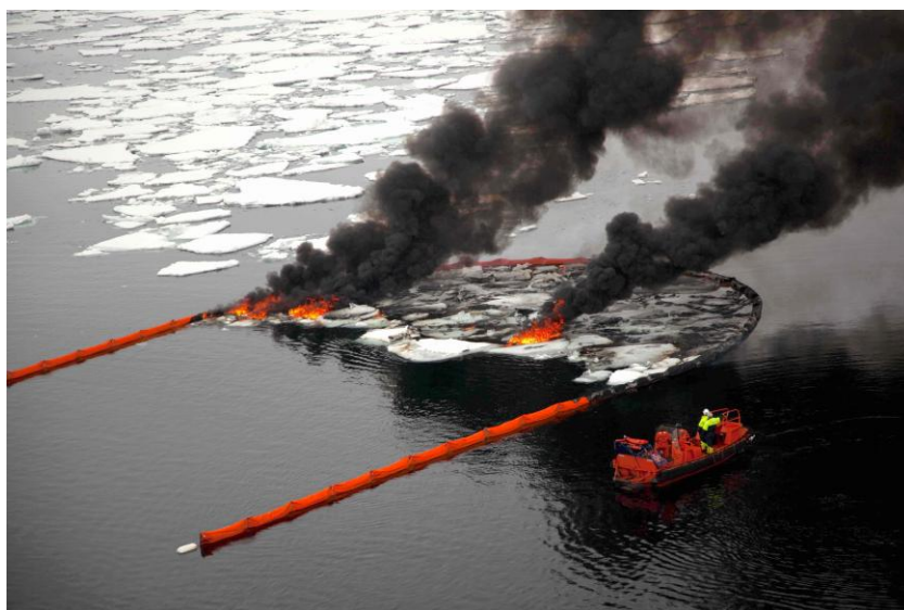
Figure 6-32. Burning crude oil spilled into a field of ice cakes collected by towing a fire boom through very open drift ice in the Norwegian Barents Sea, 2009 (Potter et al. 2010).
