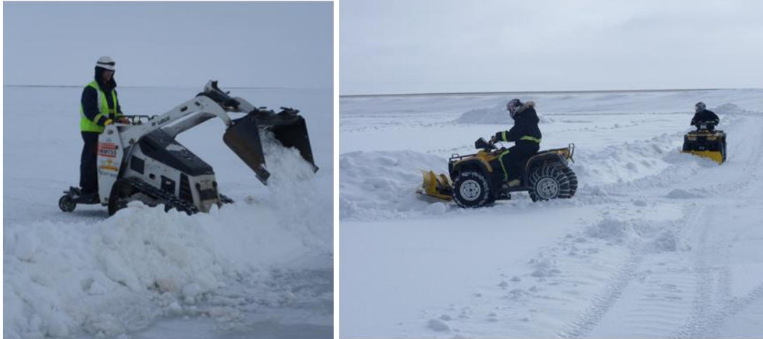
Figure 6-23. (Left) Walk-behind skid steer creating a snow berm. (Right) ATVs with plows create snow berms. Photos: ACS.
