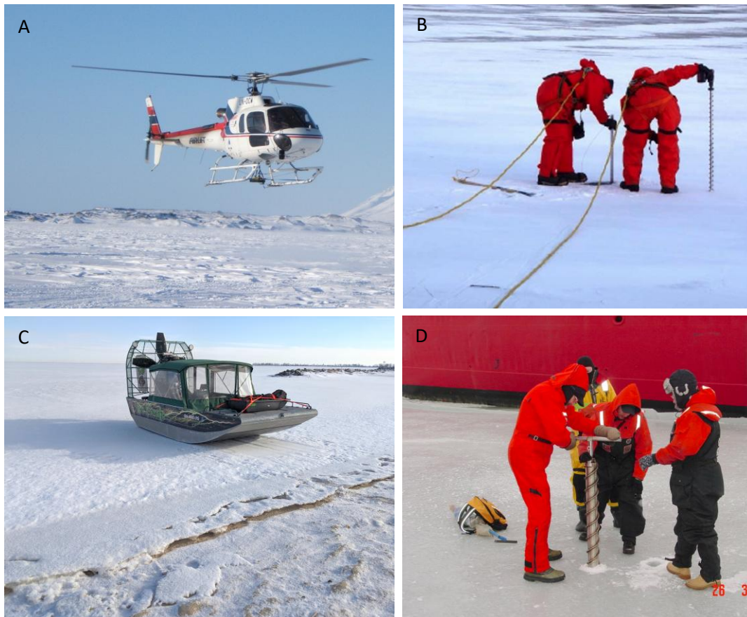
Figure 2-15. A) Profiling ice with a lightweight GPR mounted under a helicopter. Photo: D. Dickins. B) Auguring the ice to check thickness. Note the “buddy system”, flotation suits, and safety lines. Photo: Enbridge 2018. C) Air boat used for collecting samples on Lake Erie. Photo: Paul Glyshaw, GLERL. D) Ice core sampling, Green Bay, Lake Michigan. Photo: G. Leshkevich, GLERL.
