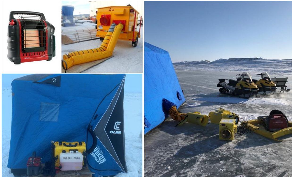
Figure 4-6. Heat options clockwise from top left. Propane heater (Mr. Buddy), industrial indirect fired heater (ES700), propane-fired shelter heater (Zumro), portable diesel air heater (Planar).
