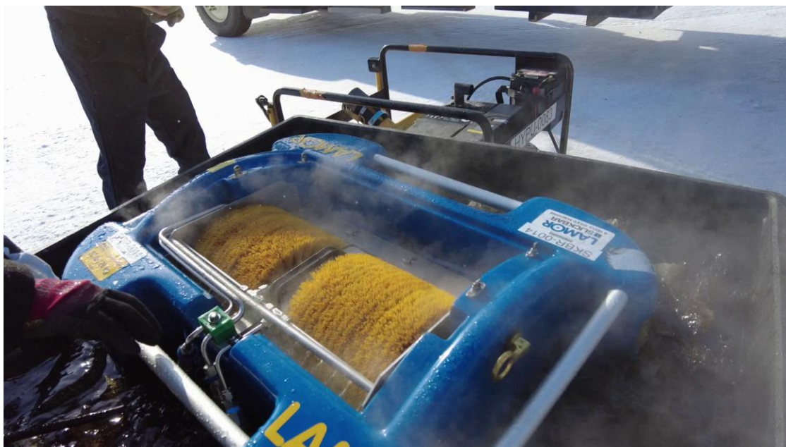
Figure 6-6. Application of steam to skimmer body. Lamor brush skimmer with steam lines. Photo: ACS.
