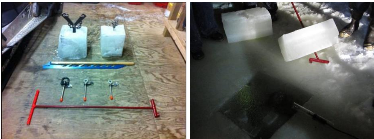
Figure 6-20. (Left) Examples of ice screws, T-bar, split-pin (or chain-linked) Lewis lifting devices, and an ice fishing handsaw. (Right) Smaller blocks may be removed using T-bars. Photos: ACS.
